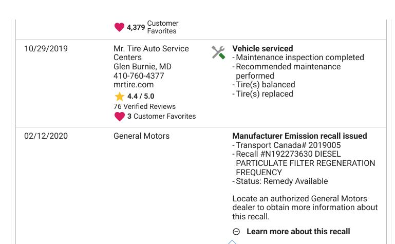
**Description:** General Motors has decided to conduct a voluntary emissions recall involving certain 2016-2019 model year diesel engine vehicles. The engine control module (ECM) in these vehicles may not adequately diagnose or illuminate the malfunction indicator lamp (Check Engine Light) when frequent regeneration of the diesel particulate filter (DPF) occurs. TBD
